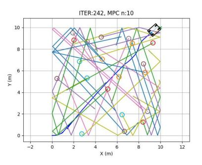
Original MPCC Time to reach the Goal: 22.1 s Collisions: 1.8 s Collision Percentage: 8.14 % Collision Speed: 0.35 m/s Calculation Speed: 0.503 s
